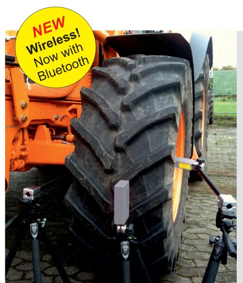
Runout Measurement Device **RPV 1300** for optimisation of the runout of large vehicle tyres.
