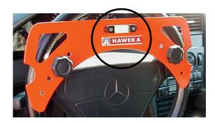
The adjustable tap on the spirit level is used on virtually all cars and light trucks.
