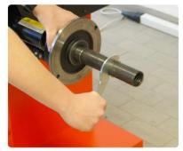
Mount a new machine connection pin (1) on the machine flange and tighten using a suitable rod.
